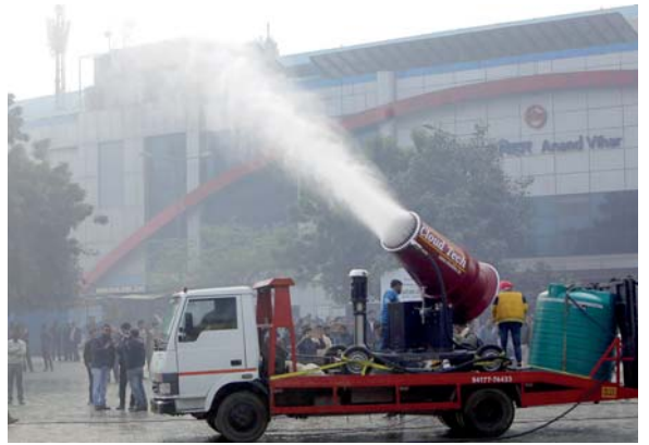
Anti-smog gun, a device that sprays water into the air to reduce pollution, being tested in Anand Vihar area of New Delhi, yesterday.
